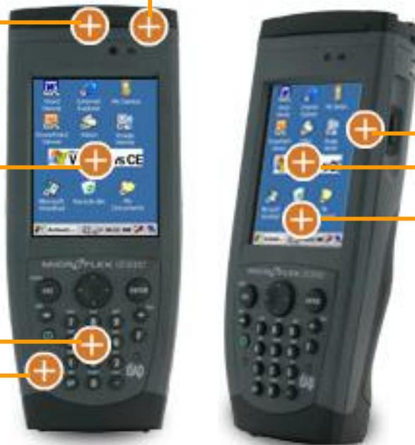
**Ambient Light Sensor** – Automatically shuts off the backlight when there is sufficient ambient light to view the screen.
