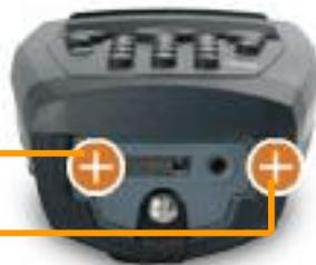
**Headset Connector** – Standard cellular phone headset can be used to listen to pre-recorded messages in a noisy environment, or to record high quality audio.
