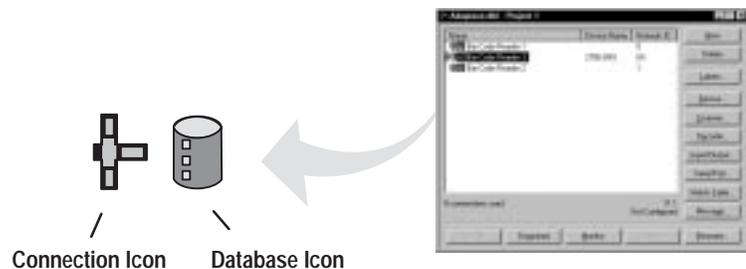
If the Reader configuration has been compared and does not match the configuration stored in the Reader, the connection icon appears red.
