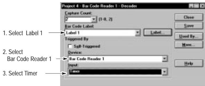
2. Select **Timer** from the Input list. Timer allows the Reader to trigger decoding without an external input (package detect). This is useful for simulating a package detector during setup.
