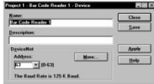
Each reader must be assigned a unique DeviceNet address. Shipped from the factory, the Reader is assigned a default node address of 63. Assign each Reader an address between 0 and 63.
