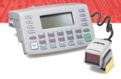
The WWC 1040 and WWC 1060 wrist computers offer powerful information gathering, processing and communications performance, yet are easy to use. They feature a programmable keyboard and backlit display, both optimally positioned for effortless keypad input and viewing, even in dimly lit environments. They weigh just 11.3 oz./316 gm and are powered by a long-lasting lithium ion battery. The ring scanner and computer are connected via an unobtrusive, lightweight cable.
