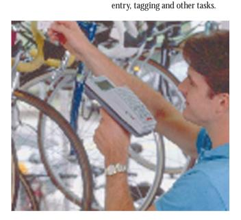
When alphanumeric input is required, the 35 - or 46-key sealed rubber keyboard enables simple and accurate manual keying. A supertwist LCD backlit display features large characters for easy reading. And, the 16-bit DOS architecture provides easy development of demanding interactive programs for retail and industrial applications.
