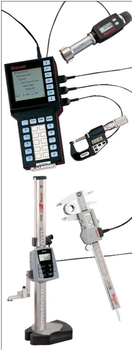
The No. 772A can simultaneously handle up to two gages, while the 772B can interface with up to eight.
