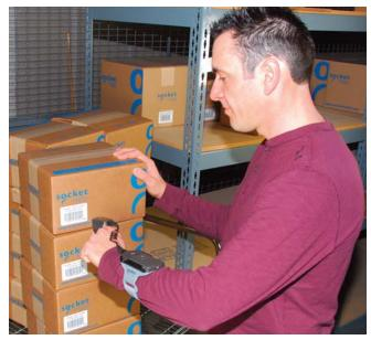
The Socket *Bluetooth®* Cordless Ring Scanner Series 9 is a wearable, hands-free barcode scanning solution that improves productivity in processes that involve repetitive scanning and package or parts handling tasks.
