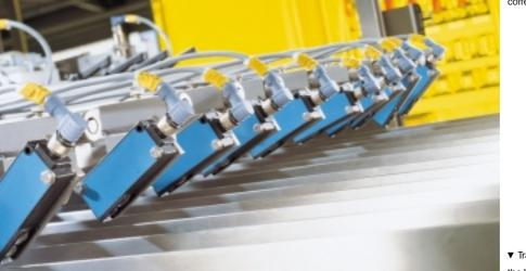
▼ Transparency poses no problems: the WL 18-2 photoelectric reflex switch monitors the edges of packaging film.
