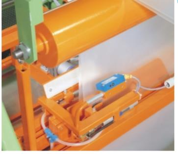
▲ Is the packaging unit complete? WT 18-2 photoelectric proximity switches provide us the answer.
