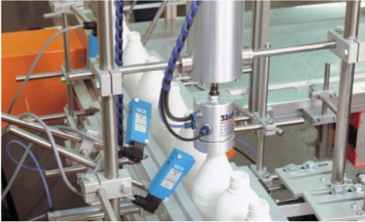
► Leak test for plastic bottles: WT 18-2 sensors used to check the presence of test objects in the automatic machine.
