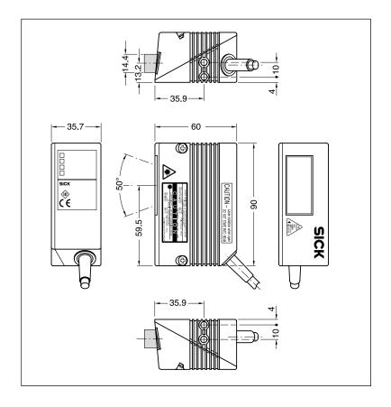
Line scanner with oscillating mirror CLV 450-6010
