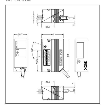
Line scanner with oscillating mirror CLV 440-6010
