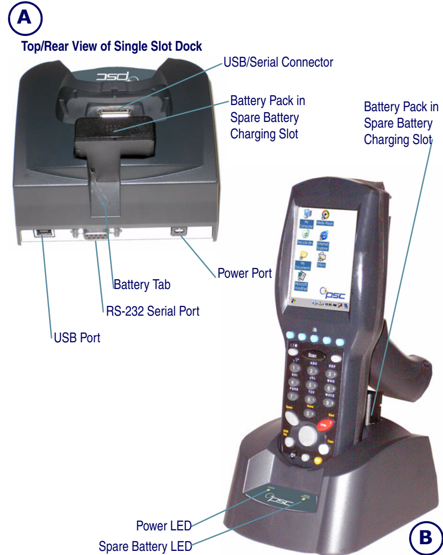
Figure 3. Charging the Battery Pack in a Single-slot Dock
