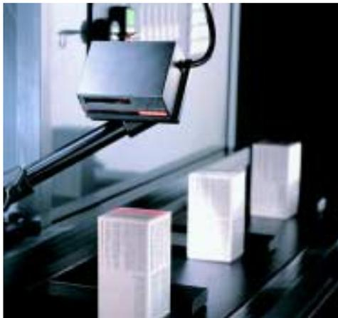
**Proprietary MS-Sensor:** Features Microscan's patented specular sensing technology that calculates why the scanner failed to read a label, pinpointing whether a label is missing or defective, or whether no
