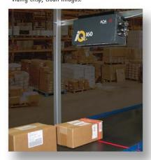
Working in conjunction with the iQ160 is an iQTroller where bar code decoding and data exchange take place with Ethernet, RS232, or optional fiber communication. A QTrace module can be added to the system providing more flexibility and functionality including dimensional data, and belt speed information. Each of these modules is enclosed in a compact, rugged housing. All this means fast and easy setup, reliable operation, and the power to aggressively read your bar codes-even under plastic.
