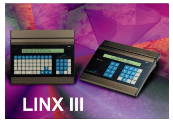
he programmable LINX III data collection and control terminals are costeffective, rugged computers, designed to collect critical data at its source. With processors, non-volatile memory, and numerous I/O device interfaces, they can be configured and programmed for a wide variety of applications such as time and attendance, access control, shop floor data collection, or machine control.
