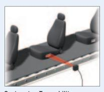
**Seat parts : Traceability**Bar codes are used for traceability management of weight, position sensors, and seat belt.
