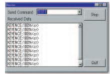
When in test mode, the BL Series performance rate (% of maximum) and reading frequency (scans per second) are clearly displayed, using built-in monitor screen.
