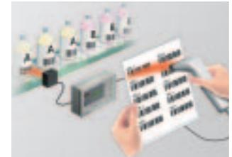
The readout bar code data can be sent directly to a PLC without any complicated communication programming.
