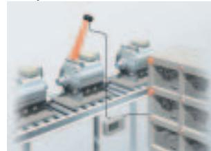
Giving directions to pick the necessary parts for compressor assembly
