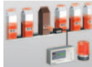
The readout bar code data is compared with the preset data, and a matched or unmatched signal can be output without a PC.
