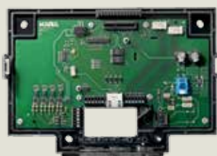
Docking station with 24 V DC
