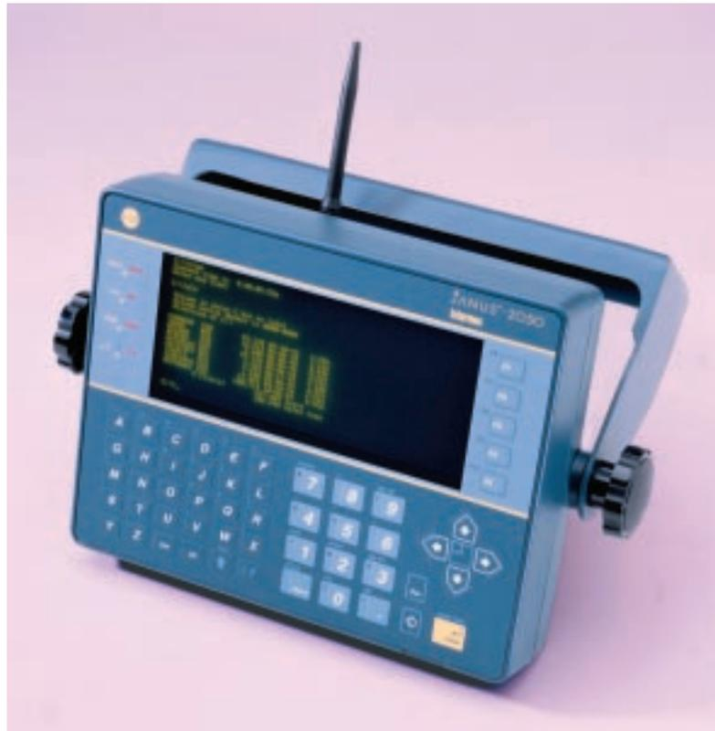
The Janus 2050 Vehicle Mount Computer is part of the most PC-compatible family of data collection products on the market. Featuring a Intel 386 processor, true MS-DOS 6.2 programmability, 4 MB of RAM, and standards-based, open architecture, the Janus 2050 enables Information Systems personnel to easily integrate a data collection system with your existing infrastructure. Plus, its broad compatibility and familiar operation can help reduce support costs throughout the life of your system.
