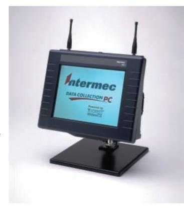
The 5055 was designed with capability in mind. The 5055 supports both 802.11b 11Mbps and OpenAir for wireless connection to your network. It supports Intermec's own wireless scanning system. The system can avoid inadvertent shutdowns and power loss with an uninterruptable power supply (UPS) on material handling vehicle. A unique recovery disk drive partition allows customers to re-image or recover corrupt drives.
