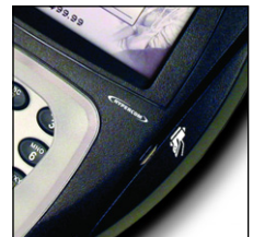
Standard dual head bi-directional magnetic stripe reader
