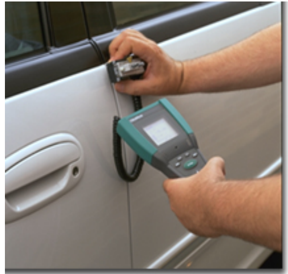
The 501 data collector with analog option can be used with an LMI gap and flush gage
