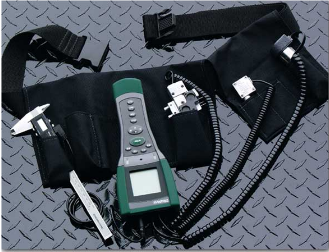
The toolbelt can hold a DataMyte 501 and a variety of digital and analog gages for roving applications
