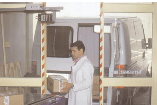
Single-cross omni-station on conveyor loading system
