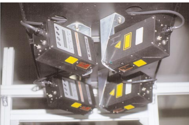
Double-cross omni-station on paired XMF-05 mounting frames
