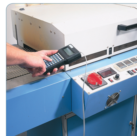
The QTERM-R55 is used to control an oven at an electronics manufacturing plant.
