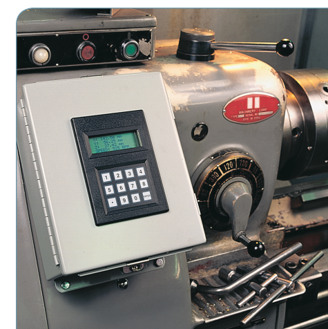
The QTERM-N15 microterminal is used in a machine shop to input and display parameters.
