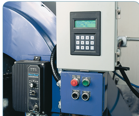
As the interface to a motion controller, the QTERM-N15 displays valuable information on the screen and allows user input.
