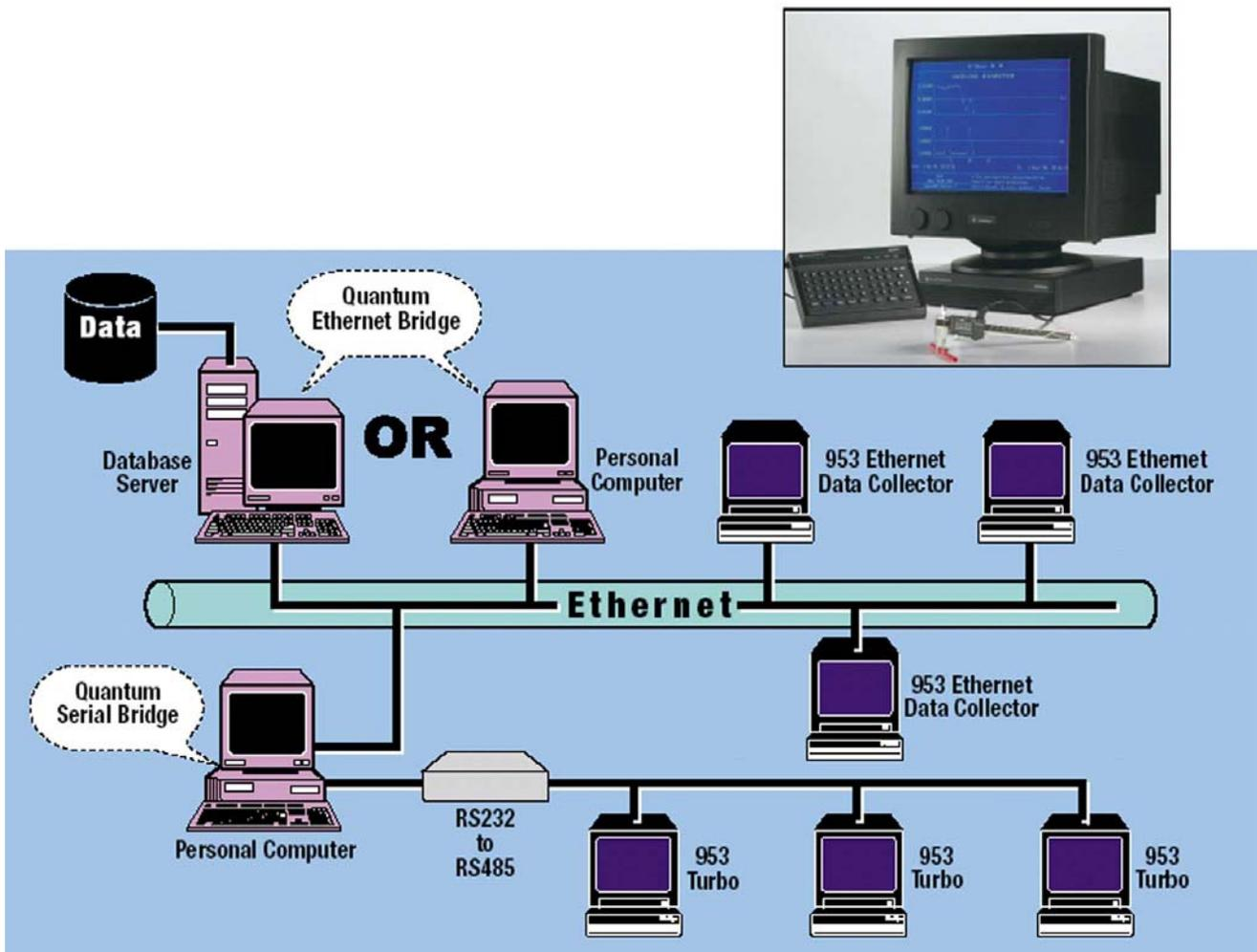
Whether you're performing on-line inspection, unattended data collection, or incoming or lot inspection, the DataMyte 953 is easily tailored to your needs. It lets you collect and analyze variables and attribute data from digital and analog gages, and from Linear Variable Differential Transformers (LVDTs). It displays a wide variety of charts, including X-bar and R, histograms, Pareto charts, and p-charts.
