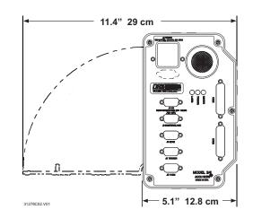
\*Communications: Programmable I/O Communication Ports RS-232, RS-422, and RS-485 Multidrop Current Loop (com1 only) DeviceNet Ethernet Profibus
