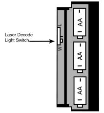
Battery Compartment with door removed
