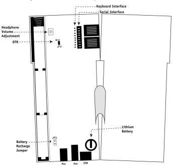
Referring to TriCoder diagram above, locate the Keyboard/Serial jumper positioned next to the two RJ45 scanner and computer ports. The jumper block is 9 positions long and has 3 rows of pins.
