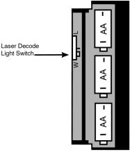
Battery Compartment with door removed
