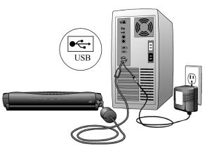
The USB symbol identifies the location of the USB port on your computer. If the plug does not attach easily, make sure that you are plugging it in correctly. Do not force the plug into the connection.
