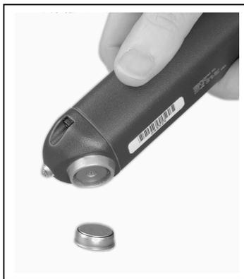
Figure 1-4 Reading a Touch Memory Button with DuraTrax
