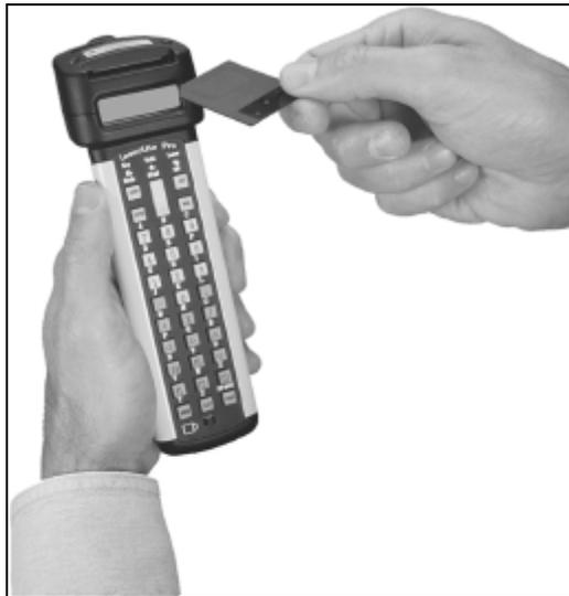
Figure 2-2 Installing Memory Card
