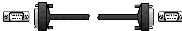
PC Serial Comm Port (DB-9 or DB-25) to Edit Suite's Computer (RS-232C) DB-9 Port
