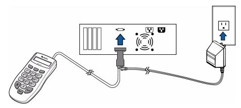
Figure 3 PINpad Device to PC/AT Cable Connection
