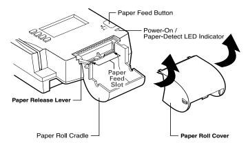
Figure 6 Thermal Printer Features
