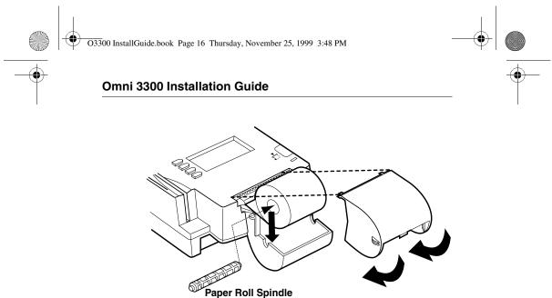
Figure 8 Paper Roll, Spindle, and Cover
