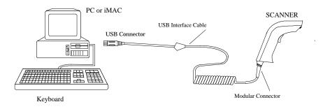
Figure 1.1. Installed as an USB Interface
