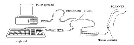
Figure 1. Installed as a Keyboard Interface
