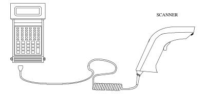
Figure 4. Installed as a Wand Emulation Scanner
