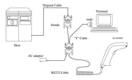
Figure 3. Installing as a Terminal Wedge
