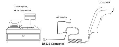
Figure 2. Installed as a Serial Interface
