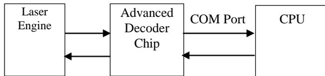
According to the above diagram, the device communicates with Decoder Chip by mean of serial port. Its communication parameter is fixed on 38400,N,8.1. Normally, the Decoder Chip is in sleep mode when COM port is not activated. When COM port is activated, the Decoder Chip will start working, and it will decode the barcode “signal” from the laser engine when the trigger key is pressed. After decoding, barcode data and its symbology type will be sent directly to the device.
