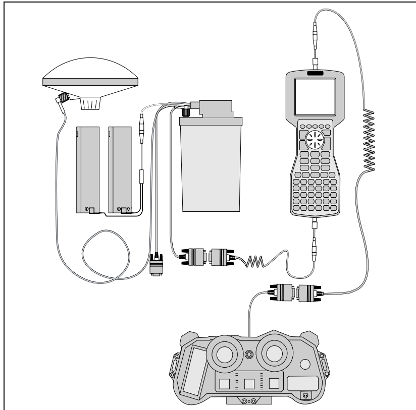
Figure I.12 LEDHA-GEO laser binoculars cabling diagram for Pro XL with TSC1
