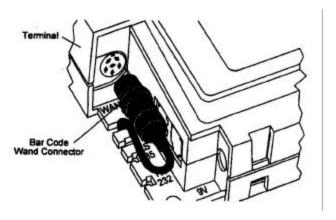
Figure 16: Bar Code Wand Connection
