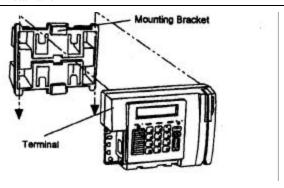
Figure 11: Terminal and Mounting Bracket Attachment
