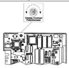
Figure 38: Display Contrast Potentiometer Location
