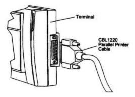
**Figure 14: Parallel Printer Connection**
