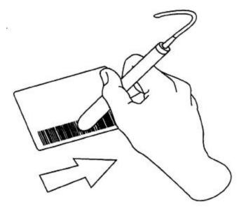
Figure 29: External Bar Code Wand Usage
