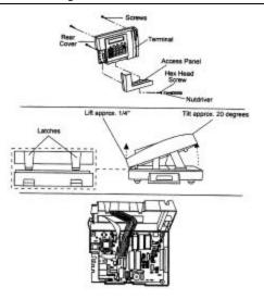
Figure 37: Rear Cover Removal
