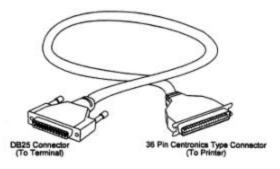
Figure 15: Parallel Printer Cable
