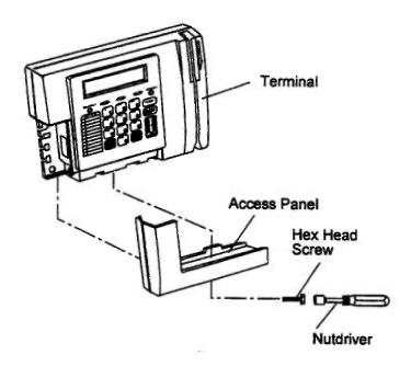
Figure 21: Access Panel Installation
