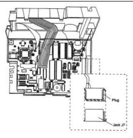
Figure 34: Internal Bar Code Reader Circuit Board Connection
