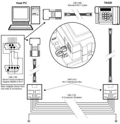
Figure 1: Serial Communication Installation
