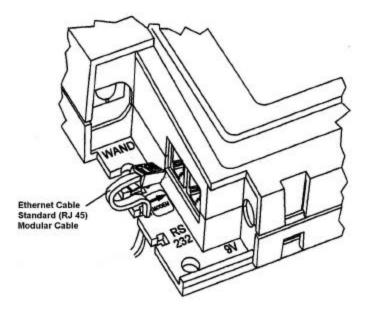
Figure 8: Ethernet Cable Communication
