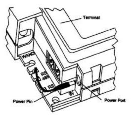
Figure 19: Power Supply Cord Installation
