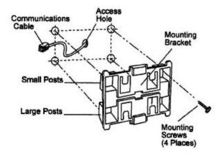
Figure 10: Mounting Bracket Installation
