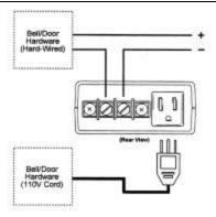
Figure 36: Signal Control Relay Wiring Diagram
