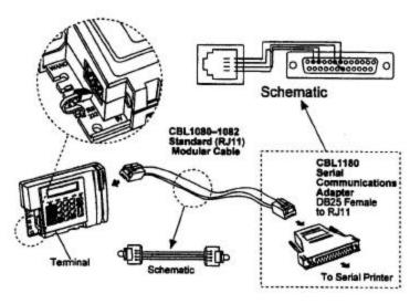
Figure 13: Serial Printer Connection
