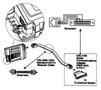
Figure 6: External Modem Communication
