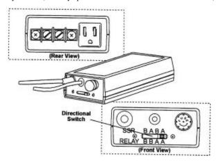
Figure 35: Signal Control Relay
