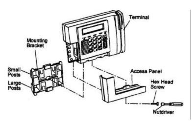
Figure 9: Access Panel & Mounting Bracket Removal
