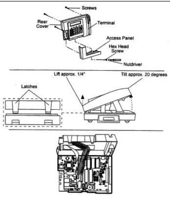
Figure 32: Rear Cover Removal
