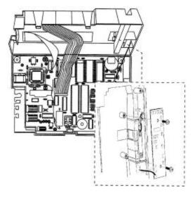
Figure 33: Internal Bar Code Reader Installation
