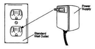
Figure 12: Power Supply Attachment
