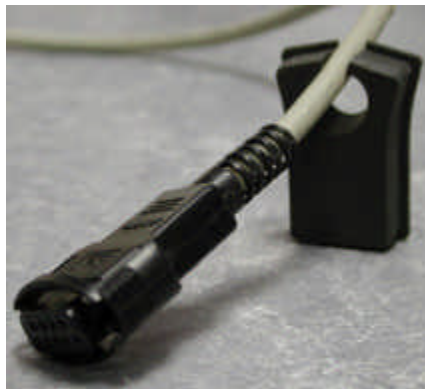
FIGURE 12 Installing the Laser Cable using a Grommet
