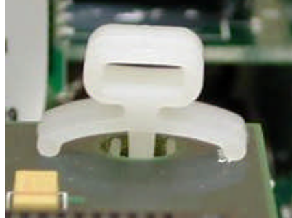
FIGURE 4 Strain Relief for Digital I/O Relay Wiring
