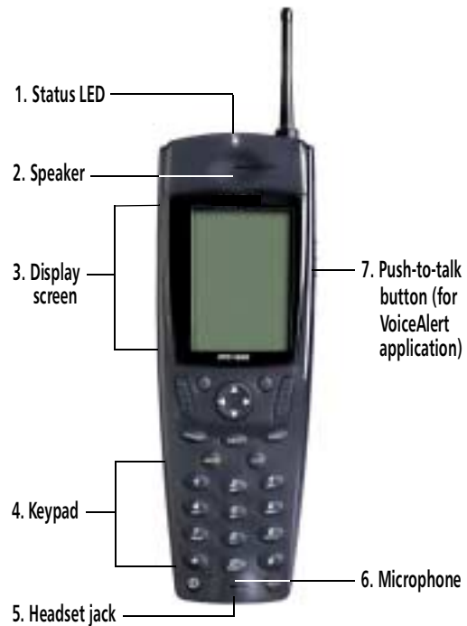
Figure 1. Parts of the PTC-1800 (front view)
