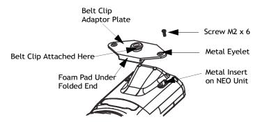
• Position the **belt clip adaptor plate** so that the thicker, folded end aligns with the angled scanner section on the back of NEO as illustrated in Figure 6.5.
