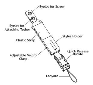
• Thread the lanyard attached to the quick release buckle through one of the accessory attachment points – the eyelets on the either side of the base of the unit. You may find Figure 6.2 useful as a reference.
