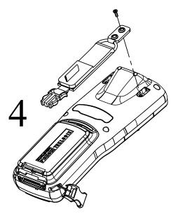
• Snap the hand-strap buckle into the lanyard quick release buckle.
