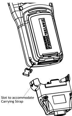
Figure 6.8 Threading Wrist Strap Through Adaptor
