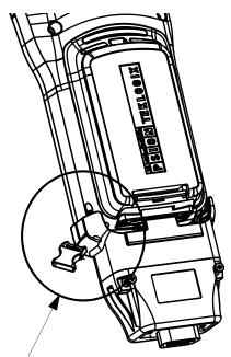
Thread Carrying Strap through slot in Adaptor
