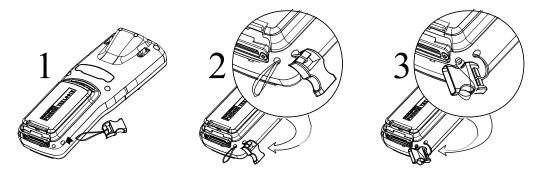
• Guide the quick release buckle through the lanyard loop to secure it to the unit.
