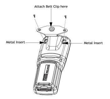
• With the adaptor plate attached to NEO, join the plastic belt clip (included in your kit) to the adaptor plate.
