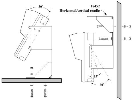
Figure 2.2 The Horizontal/Vertical Mounting Cradle
