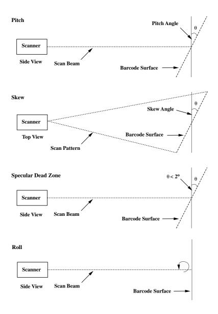
Figure 9.1 Pitch, Skew And Specular Dead Zone
