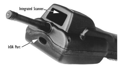
Figure 1.4 Infrared (IrDA) Port
