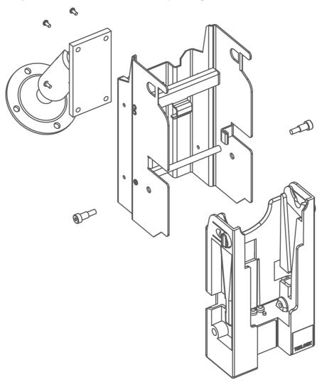
Figure 8.2 Disassembling The Cradle For Mounting
