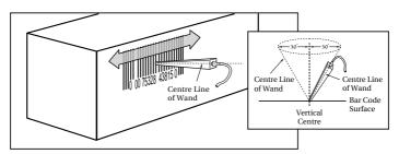
Figure 8.1 Using A Wand Bar Code Reader
