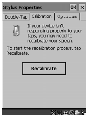
Figure 5.27 Calibrating The Touchscreen
