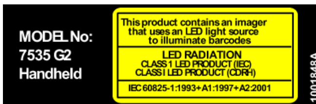
Figure 1.6 LED Radiation Notice Label
