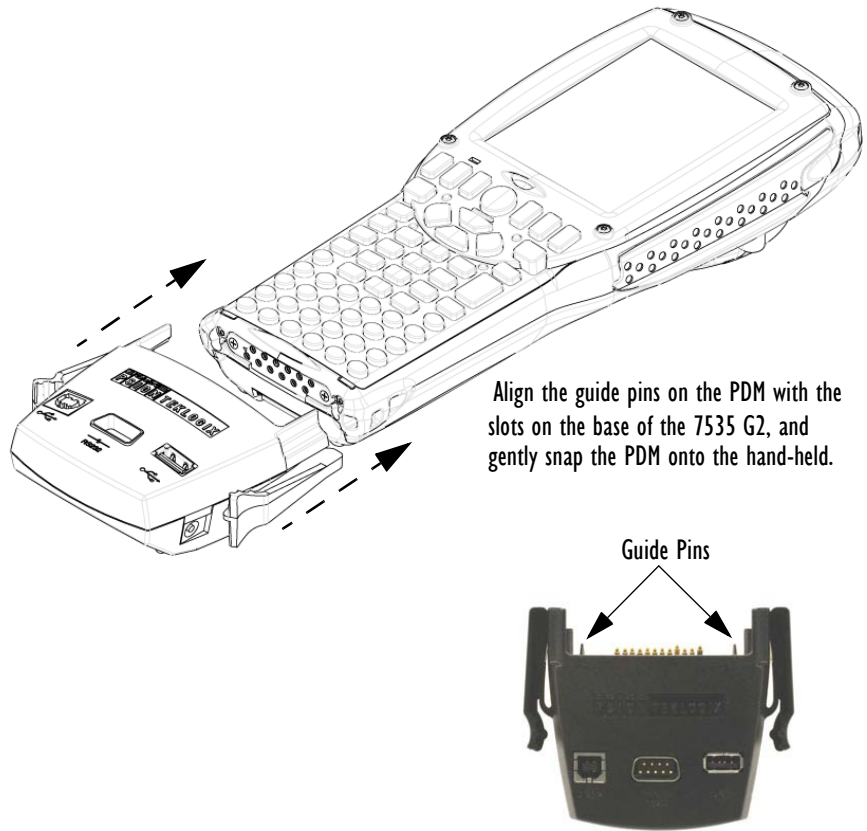
Figure 6.1 Attaching The PDM To The Base Of The 7535 G2
