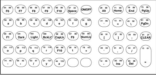
\* Functions only on units equipped with the keyboard backlight option.
