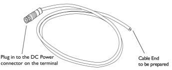
Figure 2-6. Preparing the External DC Power Cable
