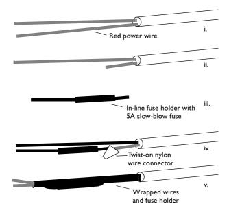
Figure 2-7. Adding an In-line Fuse Holder
