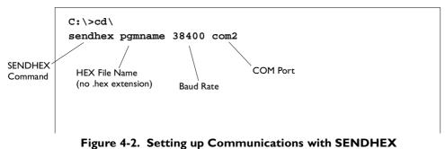
**Note:** Versions of SENDHEX earlier than version 3.0 do not support flow control. If you are using an earlier version, and errors appear, use a lower baud rate.
