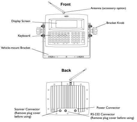
Figure I-I. Parts of a VRC 6940
