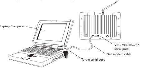
Figure 4-1. Cabling for Downloading on Benchtop
