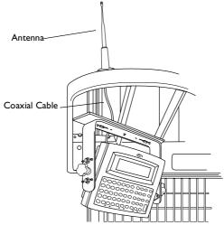
Figure 2-5. Vehicle-Mounted Antenna
