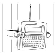
Figure 2-2. Terminal Mounted on a Wall
