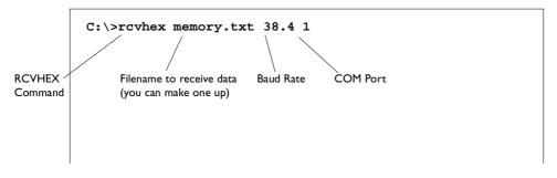
Figure 6-2. Setting up to Receive a Memory Transfer
