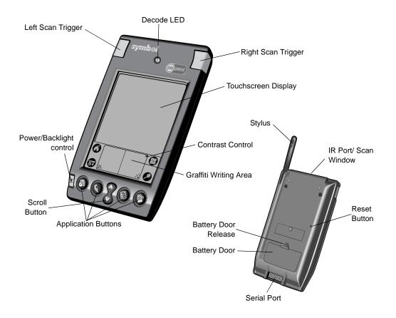
Figure 1-1. Parts of the SPT 1550
