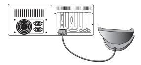
Figure 1-2. Connecting the Cradle
