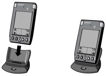
**Tip:** The curved edge on the bottom of the SPT 1550 terminal should align smoothly with the cradle when it is inserted properly.
