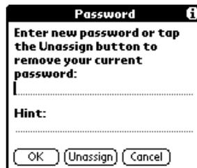
4. To change the password, enter the new password and tap the OK button. To delete the password, tap the Unassign button.
