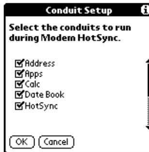
4. Tap the check boxes to de-select the files and/or applications that you do *not* want to synchronize during a modem HotSync operation. The default setting is to synchronize all files.
