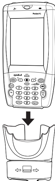
Figure 4-19. Attaching the Terminal to the Magnetic Stripe Reader
