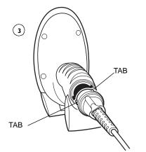
Push the boot into the scanner and twist the boot clockwise to lock into place.
