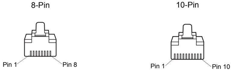
Figure 2-5. 8-Pin and 10-Pin Connectors
