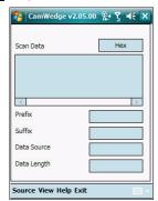
The Test window includes a button to toggle the data capture format between hexadecimal and text and a menu bar with all of the CamWedge functions.
