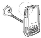
5 Connect the charger cable to the device and connect the other end of the charger cable to the cigarette lighter socket.
