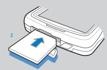
3 To remove the SD/MMC card, push down on the card and release. The card ejects from the slot.
